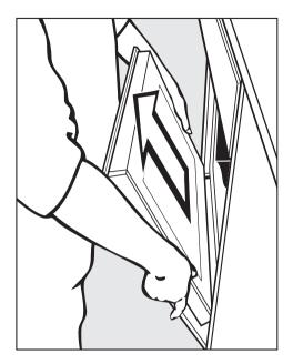
■ Hold the door securely at both sides and lift upwards off the hinge guides.
